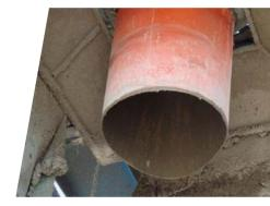
**Truckflex**<sup>®</sup> – The patented two layer hose with cutresistant outer layer and wear-resistant inner layer!
