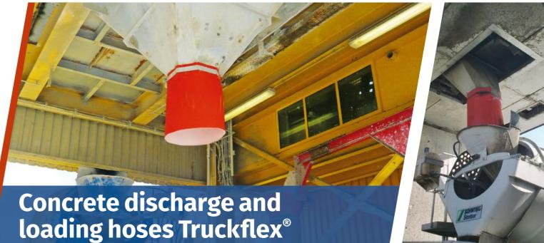
The **seamlessly fabricated** hose is highly flexible and rotatable. It is nevertheless impressive thanks to high dimensional stability. The two colour system safeguards the process via wear progression detection. The harder outer layer prevents cut injuries due to fastening clips or damaged inlet hoppers of truck mixers. The softer inner layer provides proven protection against abrasive loads.
